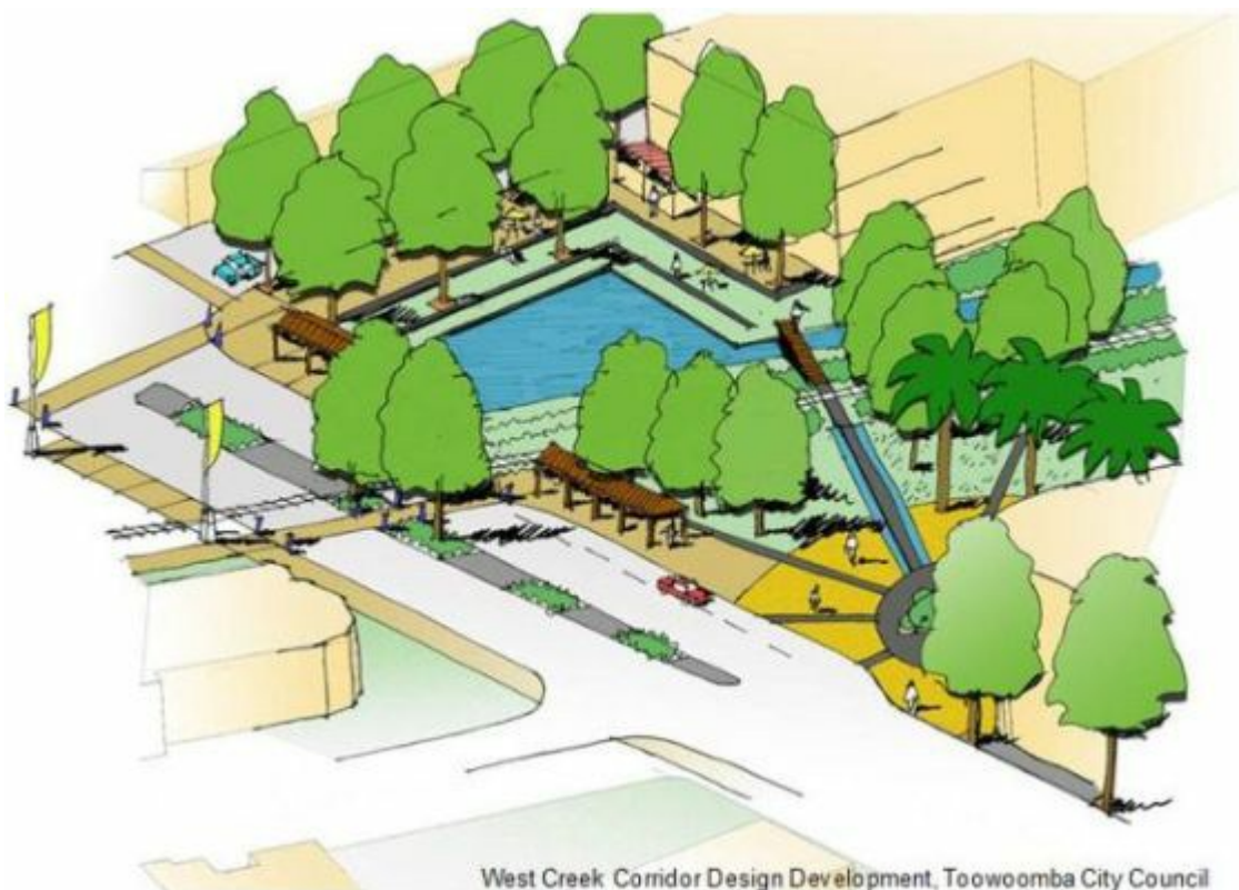
Figure SC6.4.3.9.11 Swale treatment in civic space
